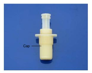
To extrude the sample, hold the 5035 Sampler with the cap pointing up to prevent spilling of the soil, then remove the cap. Hold the sampler like a syringe and push the plunger top with your thumb.
